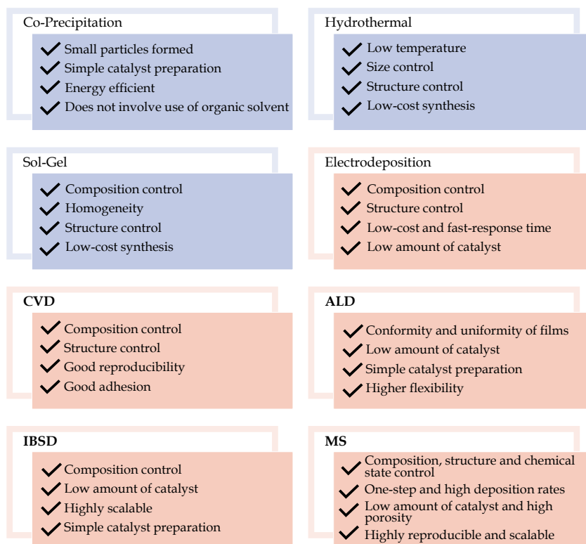
Figure 1.7. Summary of the main advantages of the catalyst deposition processes regarding their implementation in AEMWE.
