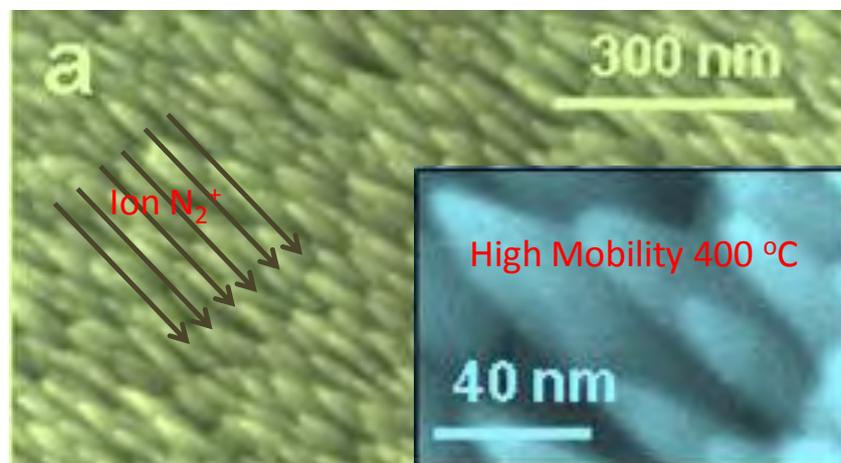
Title: Surface Nanostructuring of TiO<sub>2</sub> Thin Films by Ion Beam Irradiation.
